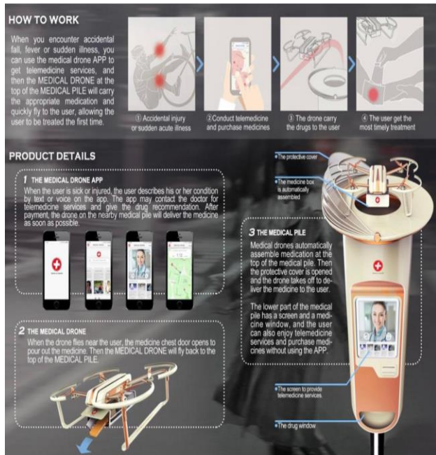
Figure 8: Working of the medical drone.
